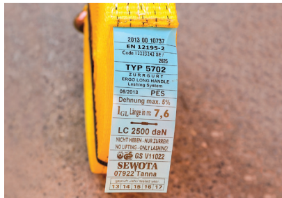
Suitable tension straps (2,500 daN) with blue label
